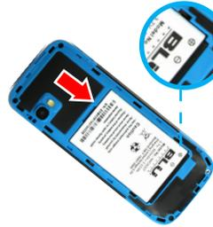
**2** To insert the battery, simply ensure the gold contacts on the battery match up with the gold contacts on the phone. Snap the battery into place.
