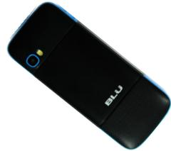
**3** Replace the back cover, ensuring the sides are all clipped into place.
