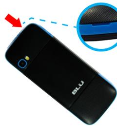
**1** Place your finger in the recess at the top of the device, and carefully lift to open the back cover.
